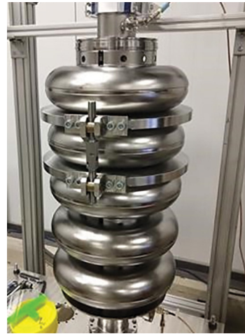
Figure 5.7: Upgrade cavity installed on the tuning stand for bead pull measurements and field flatness tuning.
